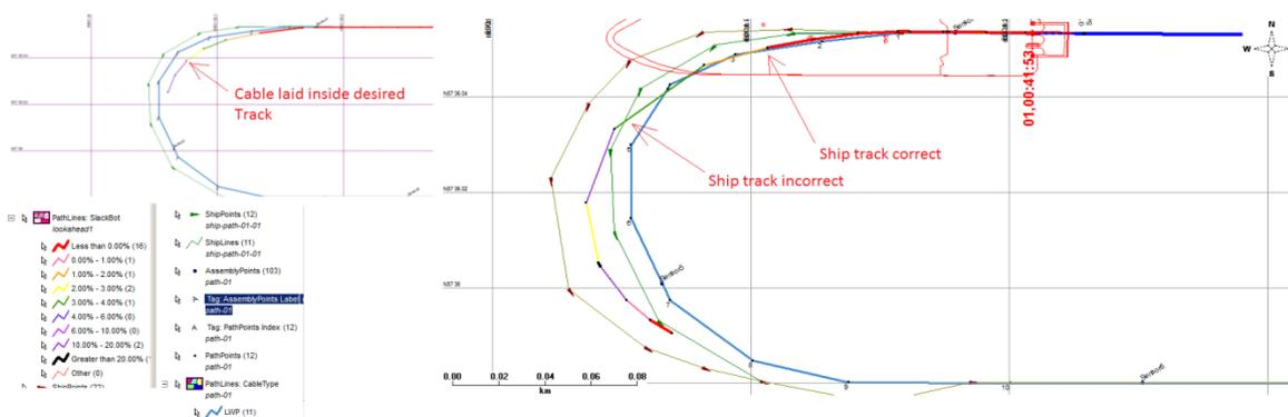
**Figure 1 Using pre-lay planning to design the correct path for the vessel**
