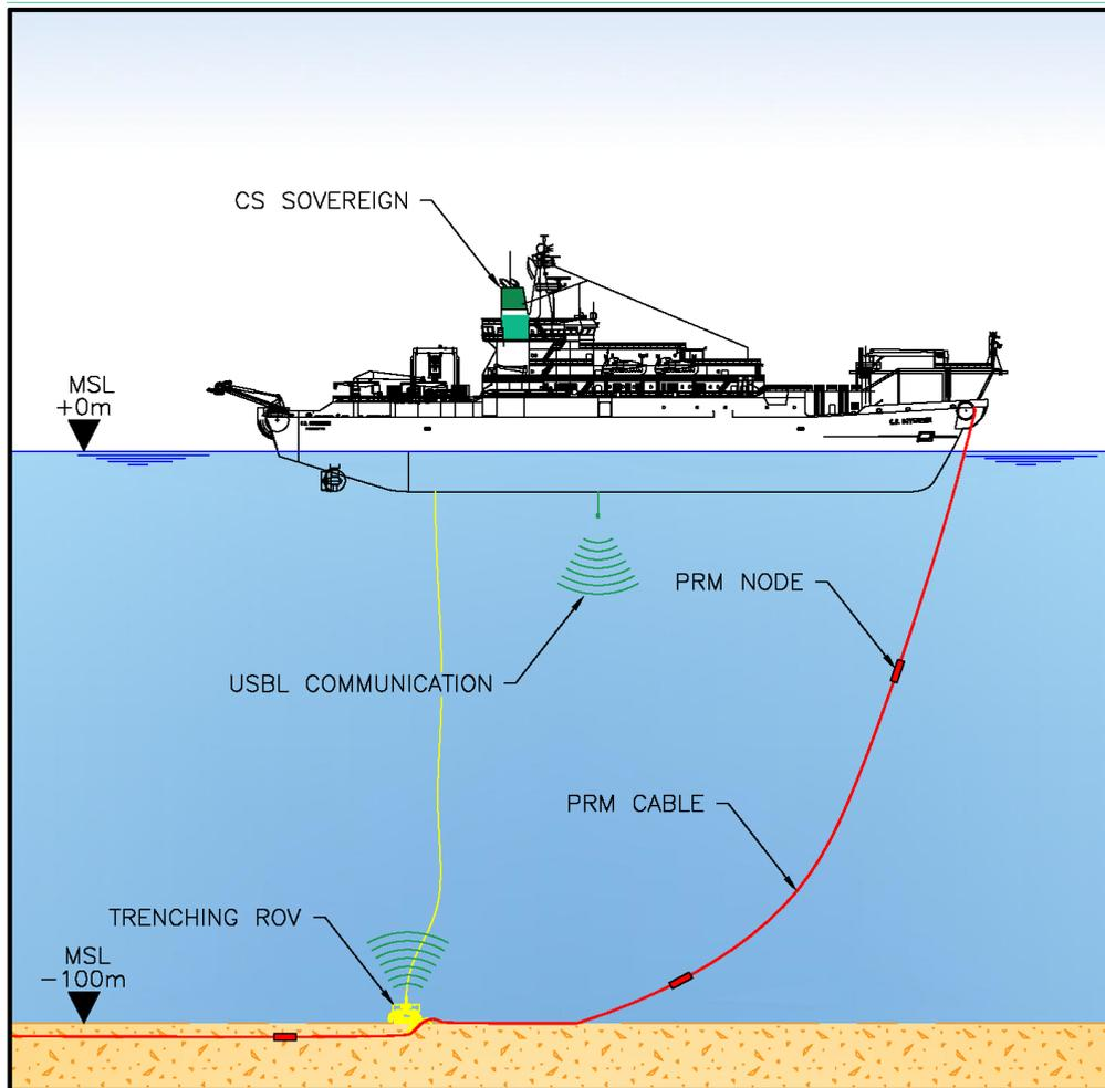
**Figure 2 Graphical representation of simultaneous lay and burial of cable**
